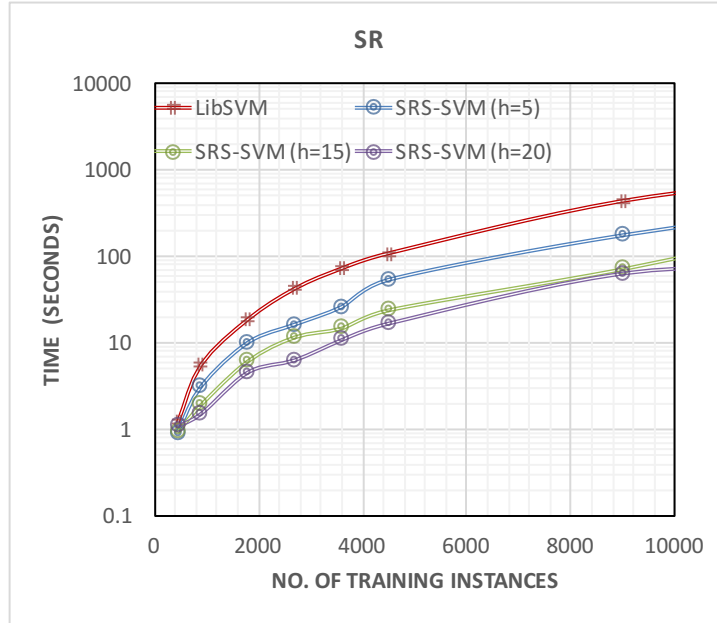
Figure 5-13: Comparing training time on SR (Shooting Range) dataset. Different number of samples are generated from the dataset and training set size vs training time plots is shown for different dataset sizes with number of subclasses ( h ) as 5, 15, and 20. Consistently, SRS-SVM takes less training time compared to LibSVM. As the parameter h is increased, the training time is observed to reduce significantly on the logarithmic scale.
